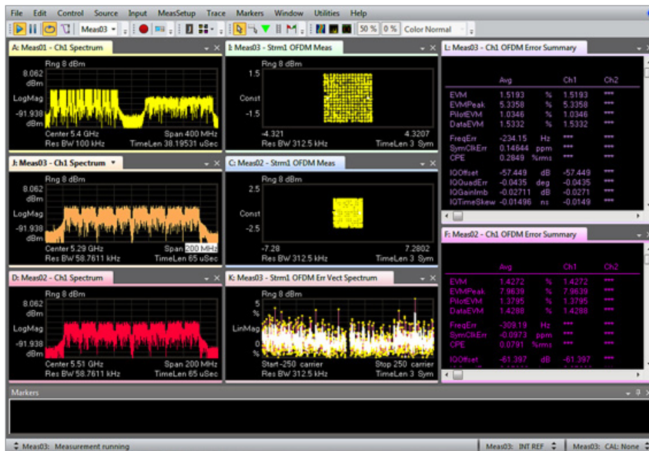
Figure 3. The Z9070B is downconverting two 802.11ac signals (160 MHz bandwidth each) that are adjacent to each other. The 89600 VSA has multi-measurement capability to analyze both signals simultaneously. Note span of 400 MHz.
